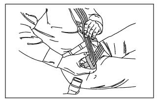
For the center rear position, if the belt stops before it reaches the buckle, tilt the latch plate and keep pulling until you can buckle it.
